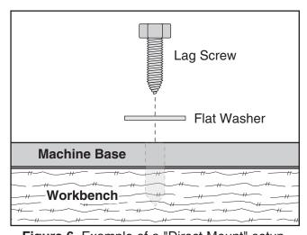
**Figure 6.** Example of a "Direct Mount" setup.
